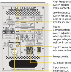
Low Frequency switch for use with subs or to simulate smaller speakers. Room Compensation switch adjusts bass when speakers are placed against walls or in corners. Input Trim control sets volume level. Power switch.
