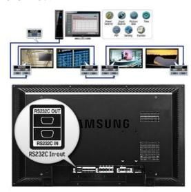
RS232C, a standard of serial communication, is used for the communication between PC and displays. Therefore, A Multiple Display Control (MDC), helping various displays to be easily and simultaneously operated on PC, is possible with RS232C function.
