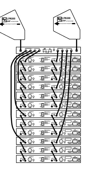
Figure 4 Antenna Chain with APD4-B
