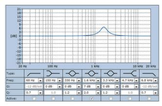
LC3-UC06E specified active equalization required for EN 54-24
