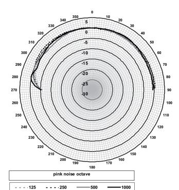
LC3-UC06E horizontal/vertical polar diagram (low frequency). Normalized at 0-degrees axis
