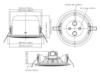
Mechanical diagram LC3-UC06E and LC3-CBB
