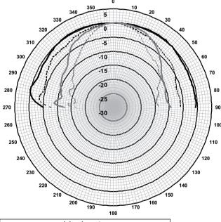
LC3-UC06E horizontal/vertical polar diagram (high frequency). Normalized at 0-degrees axis
