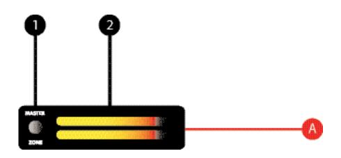
**1. Meter Switch:** Switches the display of the Level Meter (#2) between Master or Zone output signals.
