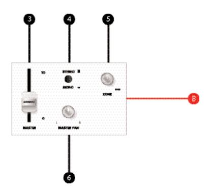
**3. Master Level:** Controls the overall output level of the audio signal sent through the Master connectors (see Output Connections.)
