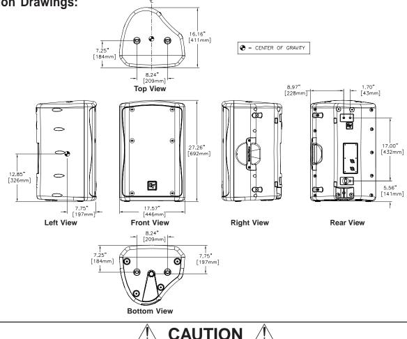
This Zx5 Loudspeaker should be suspended overhead only in accordance with the procedures and limitations specified in the *Zx5 Users Manual* and possible manual update notices. This system should be suspended with certified rigging hardware by an authorized rigging professional and in compliance with local, state, and federal overhead suspension ordinances.
