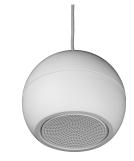
The Apart EN-SPH5T16-W is a compact 5" sphere loudspeaker with ABS housing (UI94 HB) (RAL 9010 equivalent), equipped with a high efficiency full range speaker and a multi tap 100 volt transformer, all certified according EN 54-24. The unit has a ceramic speaker line connector block and thermal fuse.
