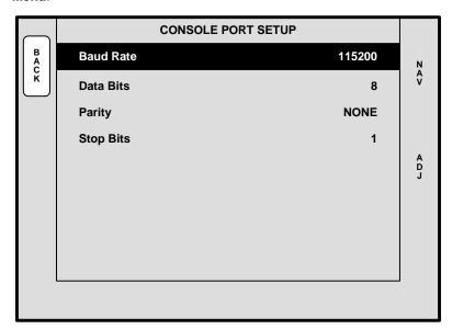
Figure 5-36. Console Port Setup Menu (sample)
