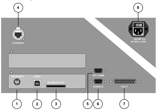
Figure 2-4. Controller Rear Panel Connectors
