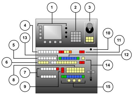
Figure 4-2. Controller SC Front Panel
