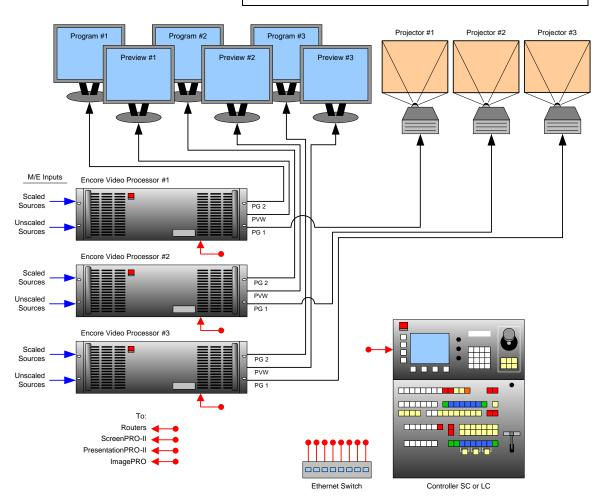
Figure 3-2. Block Diagram, Triple Screen Encore Configuration
