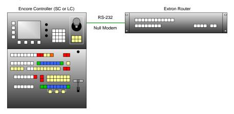
Figure E-3. Null modem configuration
