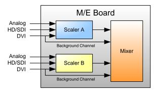
Figure 1-2. M/E Board Block Diagram
