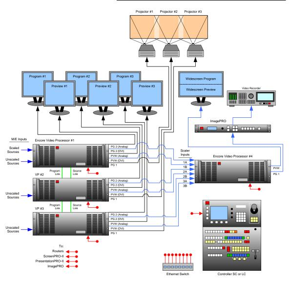
Figure 3-4. Block Diagram, Wide Screen Encore Configuration with Wide Screen Preview
