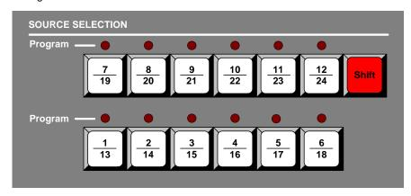
Figure 4-13. Source Selection Bus, Controller SC
