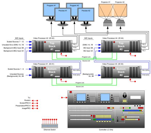
Figure 3-8. Block Diagram, Wide Screen Stack Configuration
