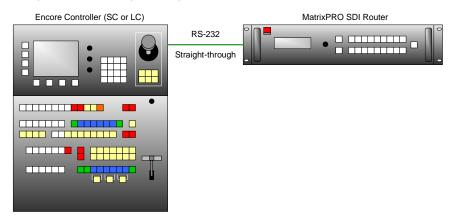
Figure E-2. Straight through configuration
