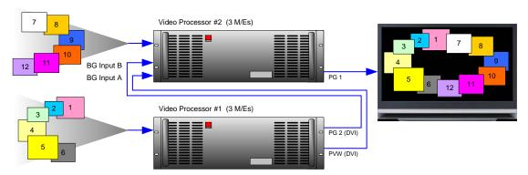
Figure 3-6. Single Screen Stack with 12 PIPs
