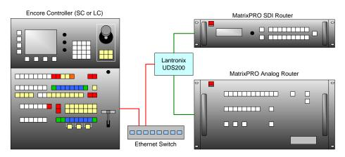
Figure E-5. Lantronix Configuration
