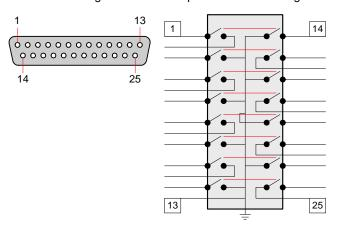
Figure A-6. Tally Connector and Circuit
