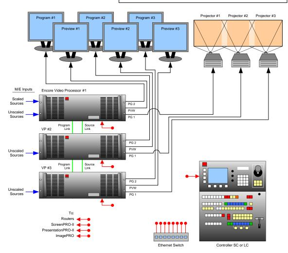
Figure 3-3. Block Diagram, Wide Screen Encore Configuration
