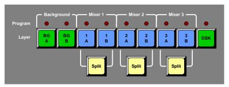
Figure 4-15. Layer Control Section, Controller SC
