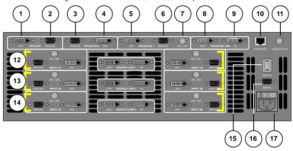
Figure 2-2. Video Processor Rear Panel
