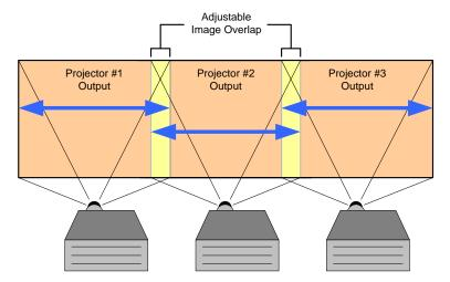
Figure 3-9. Typical three projector system
