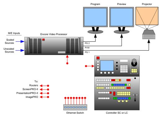
Figure 3-1. Block Diagram, Single Screen Encore Configuration
