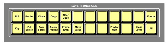
Figure 4-18. Layer Functions Section, Controller LC
