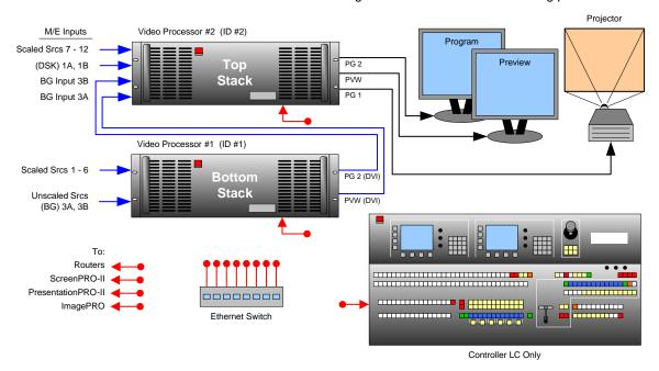
Figure 3-7. Block Diagram, Single Screen Stack Configuration
