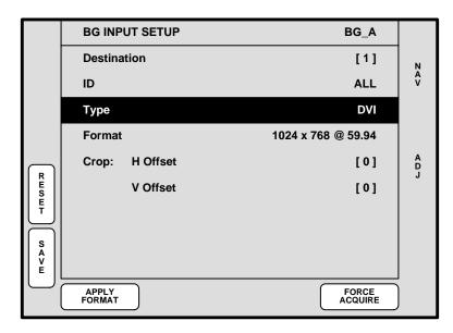
Figure 5-69. BG (and DSK) Input Setup Menu — DVI Type (sample)
