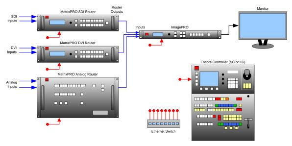
Figure D-6. ImagePRO Aux connections
