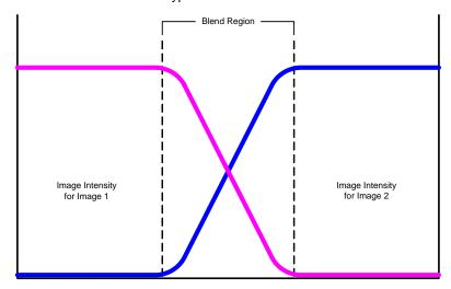
Figure 3-12. Typical Blend Function
