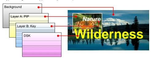
Figure 1-3. Layer Illustration — Background, Single Mixer + DSK
