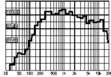
Material/Colour ABS, Polypropylene / RAL 7035 Mounting Áluminiumbracket Termination Screw terminals in termination chamber Weight 4.5 kg IP-rating 55 90°C / -40°C Max. / min. amb. temp Rated / max. power 50W / 80 W SPL 1W/1m 104 db SPL rated power 121 db Effective freq. range 140-16000 Hz Dispersion (-6dB) 1kHz / 4kHz 65° / 20° **Options** Impedance, color, label
