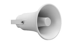
The Apart EN-H15-G is a powerful horn speaker made of UV and impact resistant ABS (RAL 7035 equivalent), (UL94V0), equipped with a compression driver and a multi tap 100 volt transformer, all certified according EN 54-24. IP66 makes it the ideal choice for industrial applications.
